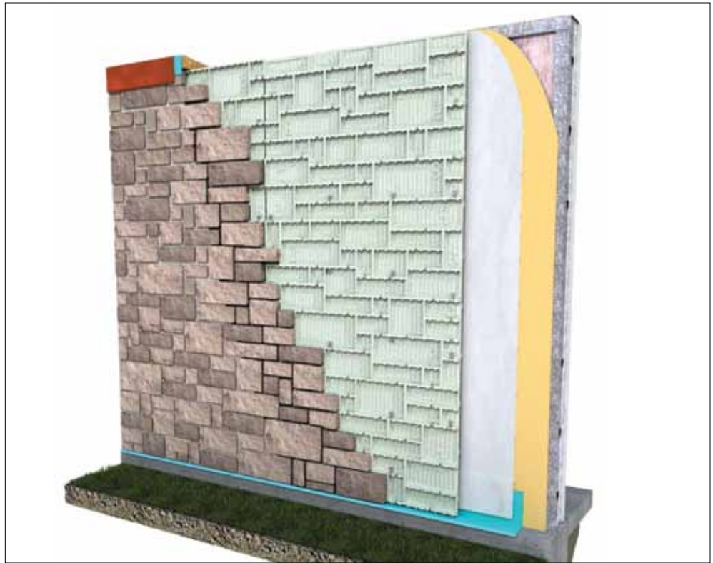
In a foam panel system, foam is applied over sheathing, flashing, and one to two layers of a weather-resistant barrier. Foam panels offer the advantage of CI, water control, and multiple patterns of face material.
