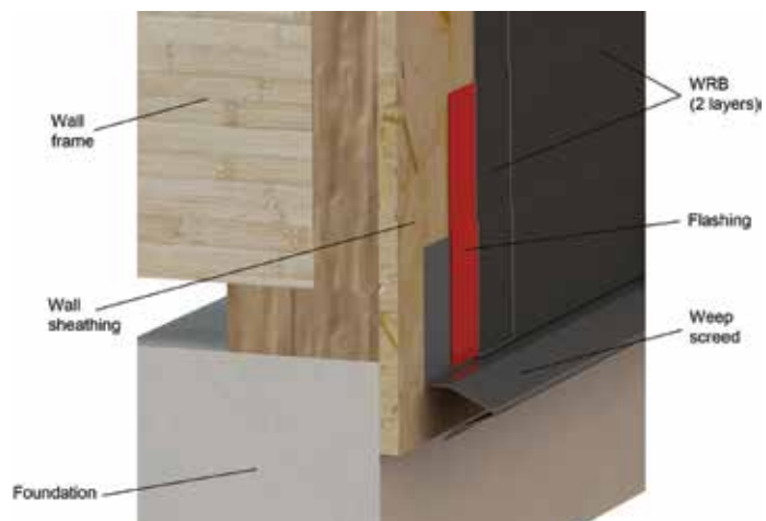
Figure 1. WRB layers overlapping flashing, and both overlapping weep screed
