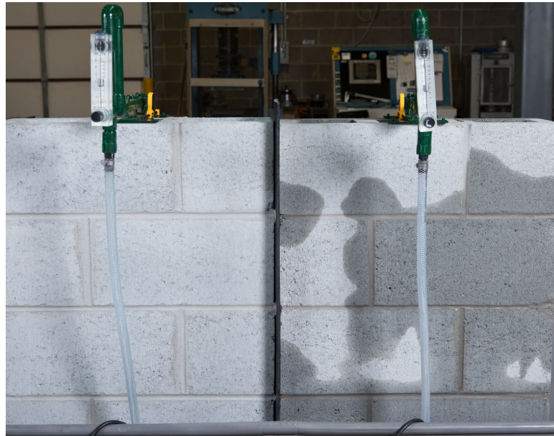
Masonry with integral water repellent mortar after 72 hours.
