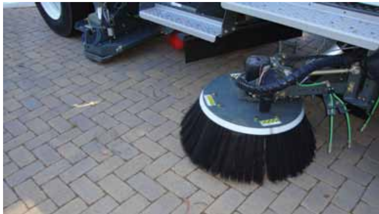
A vacuum sweeper is used at the Naval Post-graduate Facility in Monterey, California, for routine maintenance.
