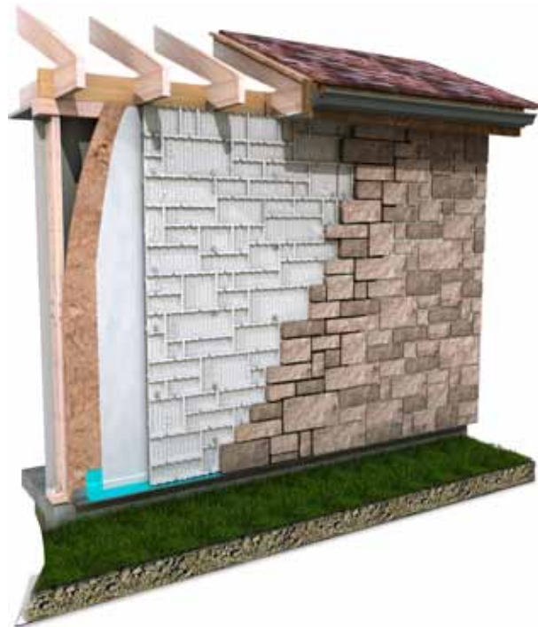
3D rendering showing the existing wall or substrate, foam insulation panel, anchor/screws, stone, and specially engineered mortar.
